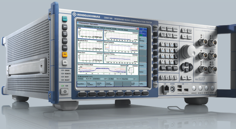
Fig. 1: The R&S®CMW500 wideband radio communication tester addresses the complete test scenario from development to production. It covers all layers and all relevant standards.
