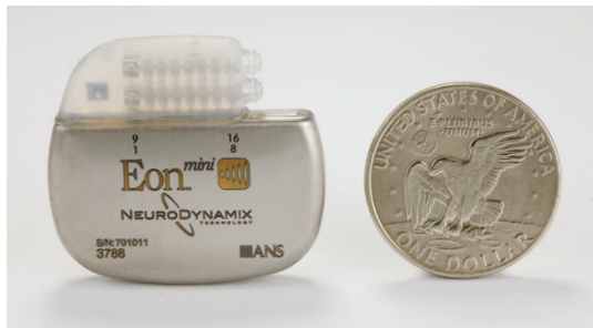
The Eon Mini neurostimulator is approved to treat chronic pain of the trunk and limbs and pain from failed back surgery. Courtesy of St. Jude Medical.
